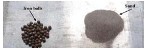
Fig. 3: Photograph of sensible heat storage materials
